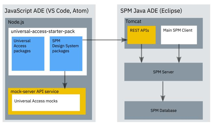
Figure 3. SPM React and Java application development environments
