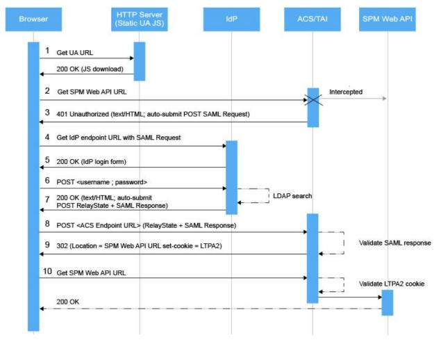
Figure 5. SP-initiated flow for Universal Access in WebSphere Application Server
