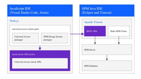
Figure 5: Universal Access React and Java<sup>™</sup> application development environments
