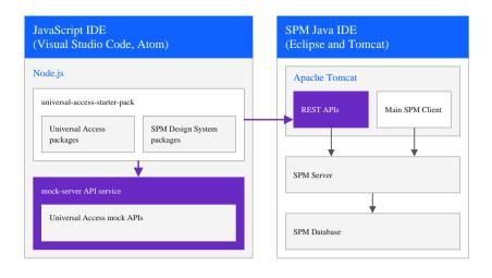
Figure 4: Universal Access React and Java™ application development environments
