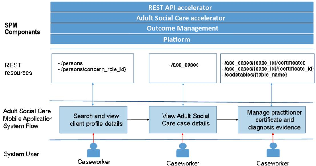
Figure 2: The Cúram REST API overview diagram
